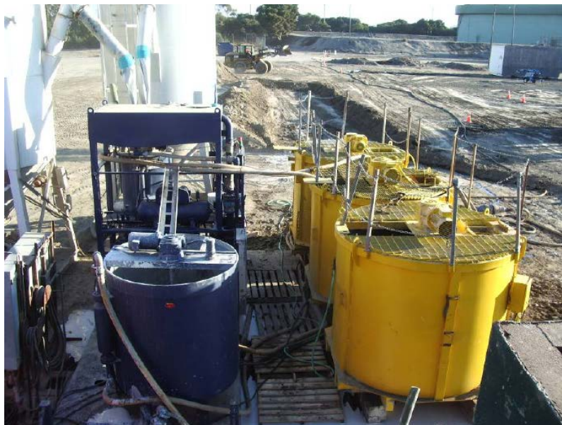
Figure 138. Photo. Slurry batching plant for larger mixing project.
