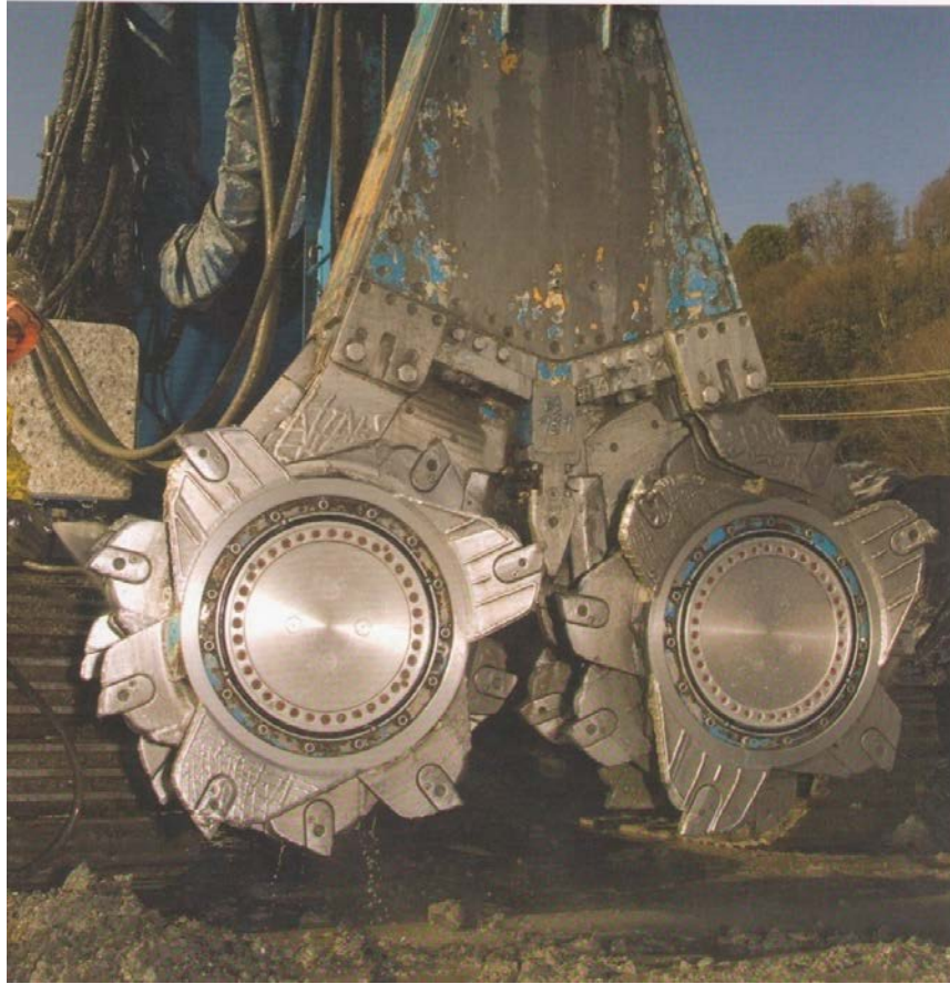
Figure 146. Photo. CSM method cutter wheels.
