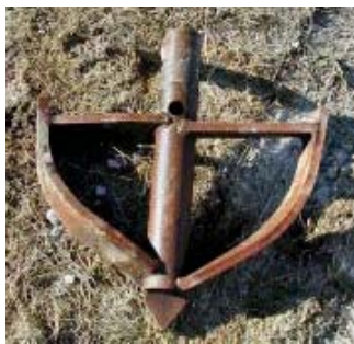
Figure 151. Photo. Typical mixing tool for DRE methods. (118)
